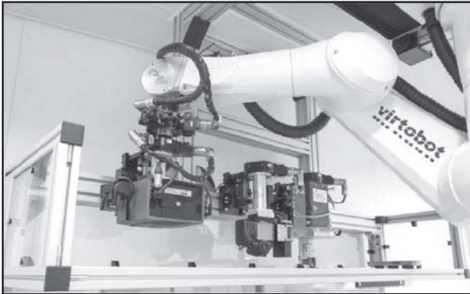
Figure 2 Tool stand during automatic tool change. Left to right: Surface scanner, digital photo camera for photogrammetry and biopsy module.
